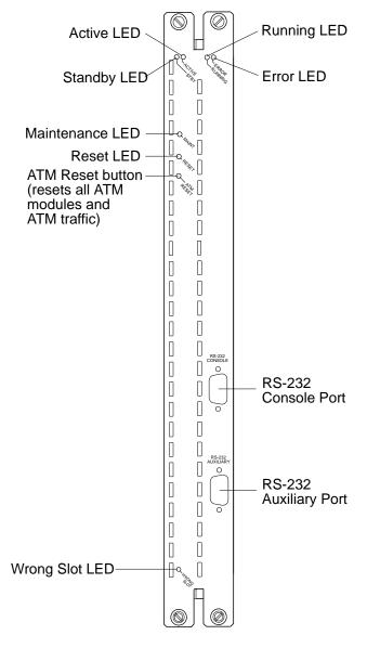
Figure 2-4. Front Panel of 6416SW Module
